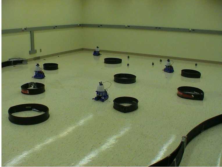
Figure 6: The environment in the communication experiments was approximately 7 m x 8 m. All experiments contained nine targets and eight obstacles. As before, the obstacles were relatively low and did not block a robot’s view of the landmarks or of each other. However, they did block a robot’s view of the targets.
