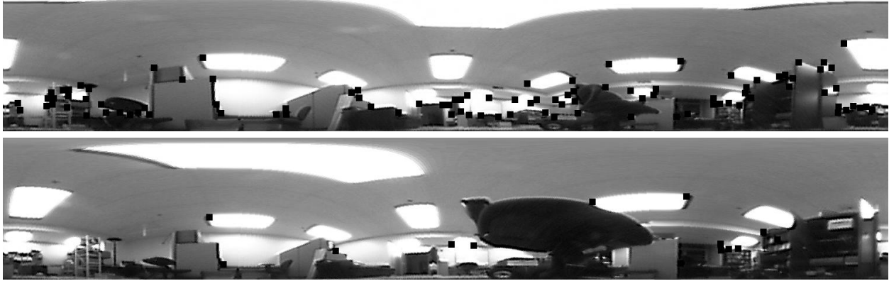
Figure 10: The 100 best features selected by the KLT algorithm in the top image are shown as black squares. The bottom image shows how many features were tracked from the top image to the bottom image (corresponding to a robot translation of approximately 0.6 m.)
