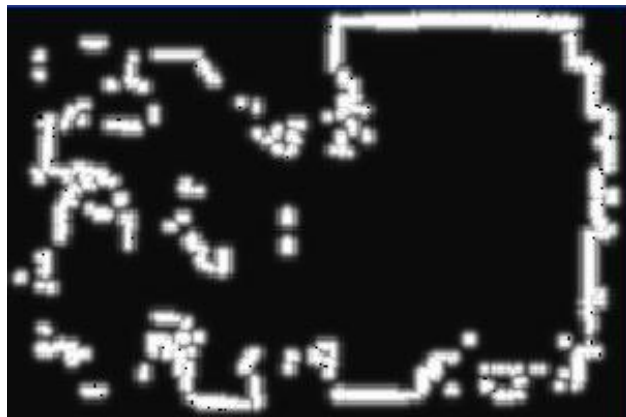
(c) Likelihood field. Brighter areas have a higher likelihood of being perceived as an obstacle.
