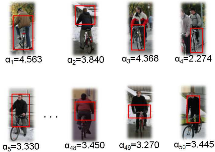
Figure 6: Several of the selected regions and confidence values (alpha) as identified by the AdaBoost algorithm.
