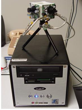
Figure 1. The CAMEO † system consists of a set of firewire cameras arranged in a panoramic fashion and a small-form-factor PC.
