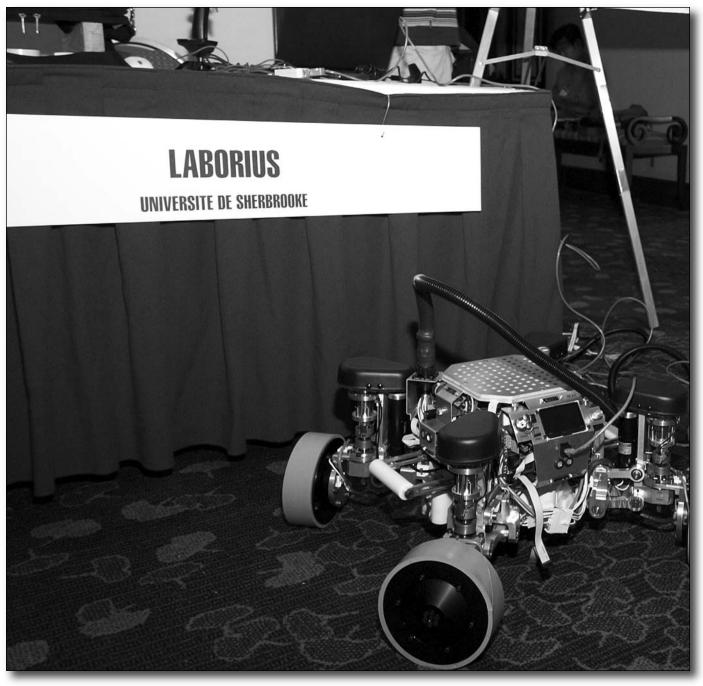
Figure 16. The Azimut-2 Omnidirectional Modular Platform from the Universitè de Sherbrooke.
