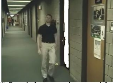
(d) Example 2: A person has emerged from their office. Their face is detected at the entryway to their door and the contiguous region represented by their door is obtained with the Grab function. The door is highlighted in white.
