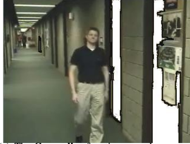
(e) The Generalize function uses the parameters returned by the contiguous region capture routine to find another door in the foreground of the image.
