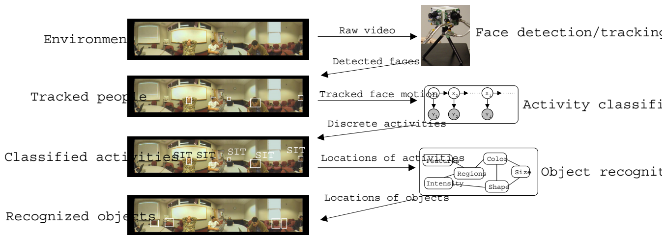
Figure 4: Flow diagram of FOCUS. In this example, an omni-directional camera captures raw video from the environment. This video is searched for human faces. When a face is found, the person is tracked over time. The motions of the individual faces are analyzed for specific activities. Finally, the “functional” aspects of the activity are used to classify “structural” features of objects used in that activity (i.e., chairs are identified where people sit).
