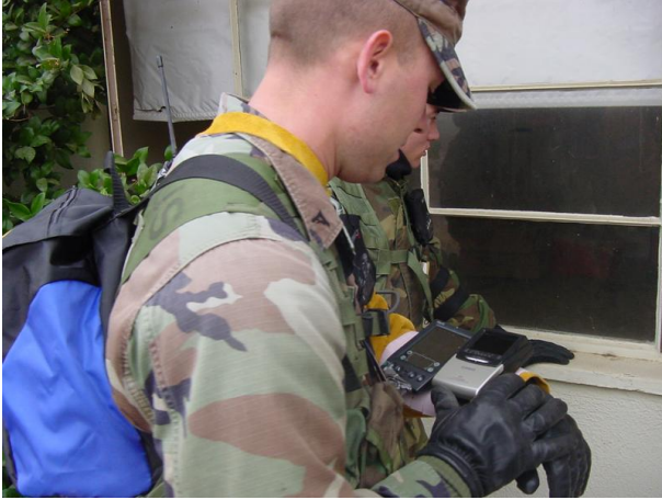
Figure 3: Operator wearing prototype PDA user interface. The monitor attached alongside the PDA on the sleeve is used to view the video from a Scout.
