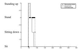
Fig. 7. Classified actions from the center person in the dataset illustrated in Figure 6. Of the 315 timesteps in this dataset, only 29 of the states were misclassified. The Y-axis represents the state where, 1="Sit", 2="Sitting down", 3="Stand", and 4="Standing up". The X-axis is the frame count. The data was captured at 15 fps.
