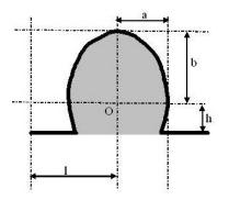
Fig. 4.  $\Omega$  shaped template for 2D projection of head and shoulder
