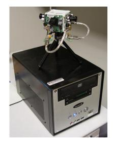
Fig. 1. The complete CAMEO system consists of several calibrated firewire cameras and a portable image-processing workstation.
