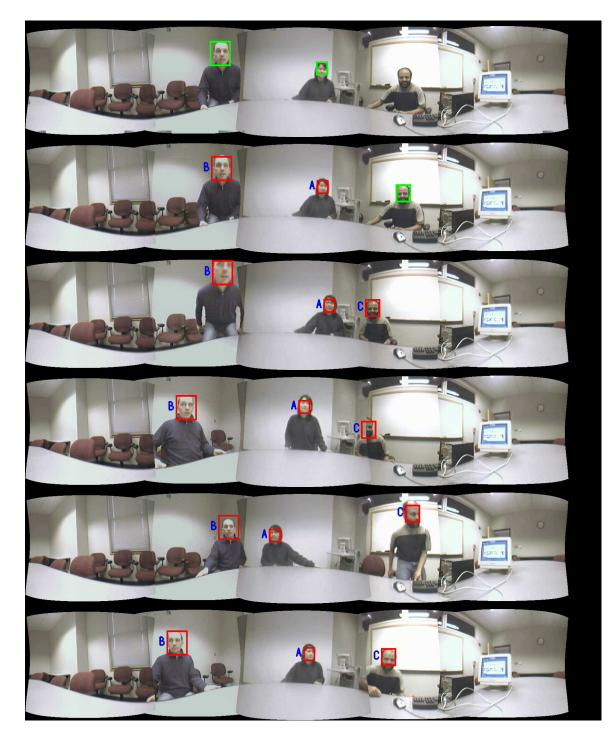
Fig. 6. CAMEO's face detection and tracking results. Frames 1,2,20,60,150, and 200 are shown above. Persons "A" and "B" were detected in frame 1 and person "C" is detected in frame 2. All three persons are subsequently tracked through the sequence.
