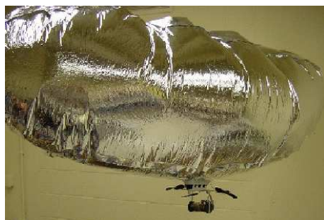
Figure 4. A Scout-controlled blimp. The fans that control the blimp’s motion are actuated instead of the Scout’s own wheels.
