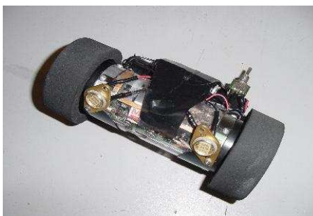
Figure 5. The IR Scout is equipped with infra-red emitting LEDs which allow the Scout’s camera to be used in complete darkness.
