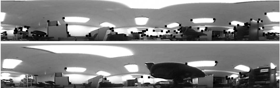
Figure 8.2: The 100 best features selected by the KLT algorithm in the top image are shown as black squares in the top image. The bottom image shows how many features were tracked from the top image to the bottom image (corresponding to a robot translation of approximately 0.6 m).
